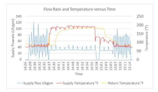
1. Supply water flow rate (gpm): This is a measurement of the flow rate of the water entering at the beginning of the circuit. It is important to note that the graph of this data shows 3 distinct sections that each pertain to one of the cleaning phases.
